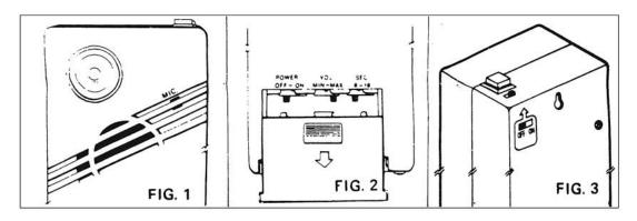
On the top of the unit has a recording button and a sensor ON/OFF switch. When the sensor ON/OFF switch is in "OFF" position and the record ENABLE/DISABLE switch is in "ENABLE" position, you can record your message by pressing the recording button. When the sensor switch is "ON" the recorded message will playback when people pass by. Please note that you can not record a message while the sensor ON/OFF switch is in "ON" position. (see fig. 3)
